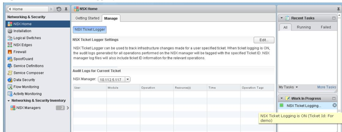
If multiple vCenter Servers are being managed by the vSphere Web Client, the ticket ID is used for logging on all applicable NSX Managers.
