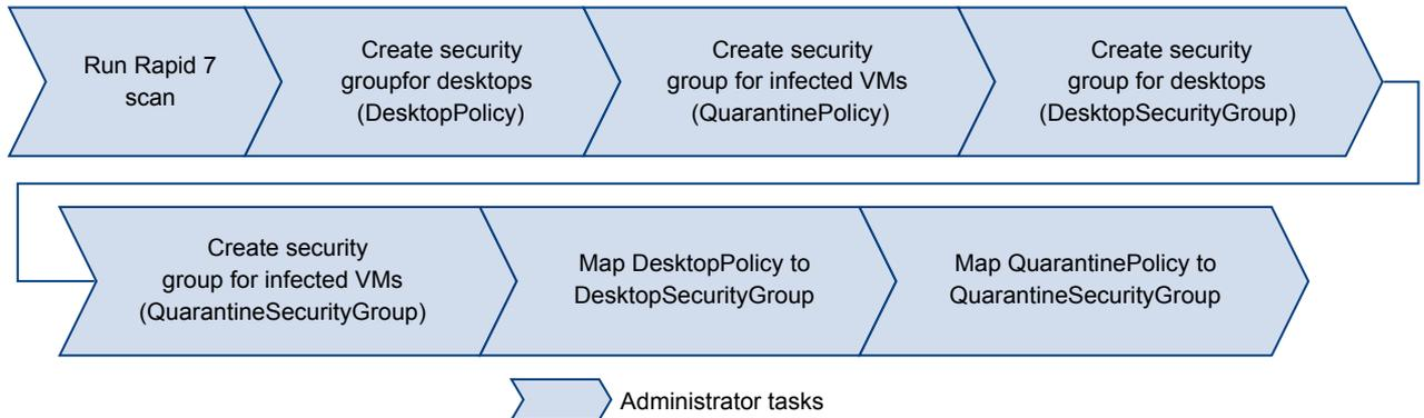
**Figure 11-7.** Service Composer Conditional Workflow
