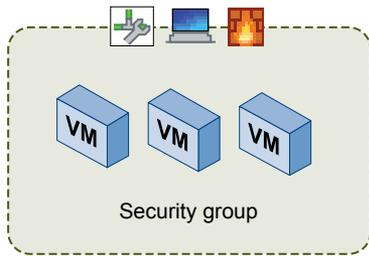
If a virtual machine belongs to more than one security group, the services that are applied to the virtual machine depends on the precedence of the security policy mapped to the security groups.
