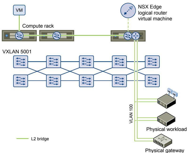
Note that you should not use an L2 bridge to connect a logical switch to another logical switch, a VLAN network to another VLAN network, or to interconnect datacenters.
