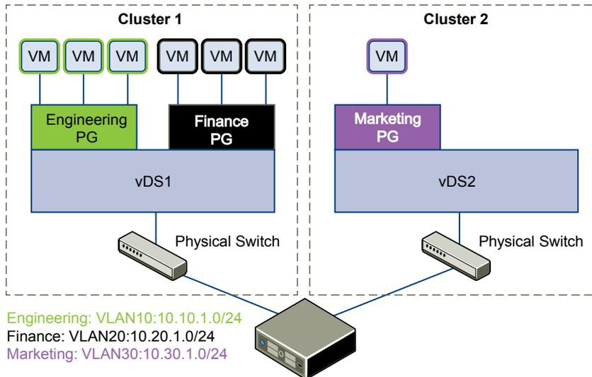
ACME is running out of compute space on Cluster1 while Cluster2 is under-utilized. The ACME network supervisor asks John Admin (ACME's virtualization administrator) to figure out a way to extend the Engineering department to Cluster2 in a way that virtual machines belonging to Engineering on both clusters can communicate with each other. This would enable ACME to utilize the compute capacity of both clusters by stretching ACME's L2 layer.
